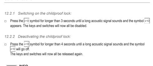
Pyrolytic ovens have a double protection system: when the childproof lock is activated, the
